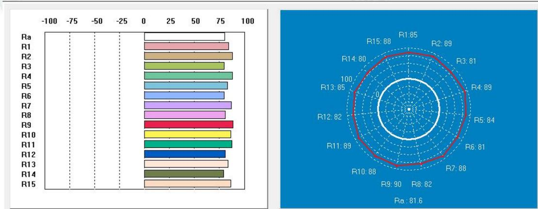
Fig 5.6 CRI histogram (left) radar diagram (right)
